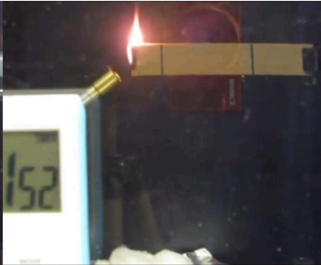
10 pph Fyrol 6 + 10% Lignin FR Additive
