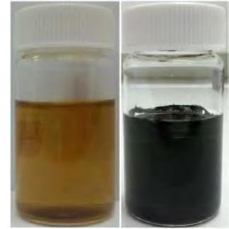
*Typical appearance of aqueous (left) and oil phases (right) from the NCW process.*
